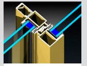
Sashes will accept glass from 4mm to 20mm thick. The ideal IGU is 16mm thick.
